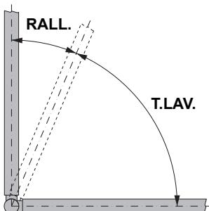
**NOTE:** with RALL. enabled (dip 4 ON), the total travel of the leaf is obtained from the total of the times set on the two trimmers (T.LAV. + RALL.).
